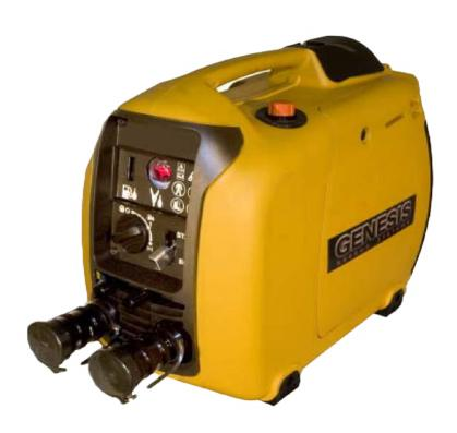
This pump features two tool "hot swappable" con- nections and two tool simultaneous use. The Eco-Silent power unit has two seperate pumping circuits that operate independently. The Eco-Silent has our patented Overdrive feature. This feature allows one tool to be used at twice the speed by combining the flow from both pump circuits into one, giving that tool more power to cut or spread. Most of all the Eco-Silent power unit is quiet with a decibel range of 63.9 to 79.6 dB at 1 meter (3.2 ft).
